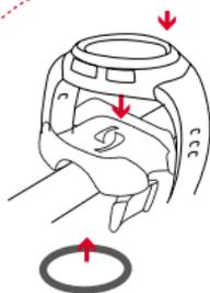
Assemble the handlebar holder.
