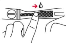
Lift the belt slightly from the skin. Dampen the ribbed zones (electrodes) on the rear of the transmitter with saliva or cardio gel.
